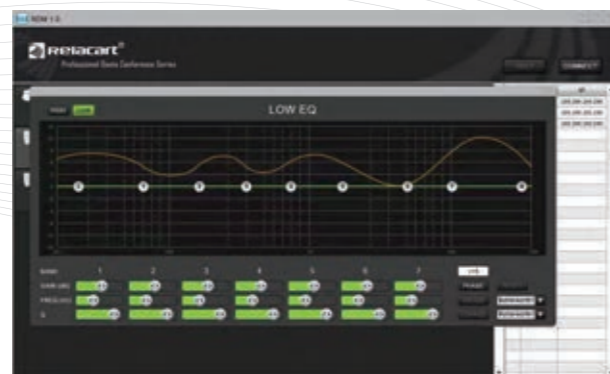
Both the tweeter and woofer can be set with 7-band equalization, high-pass filter and low-pass filter independently
