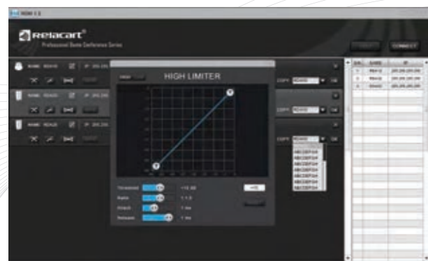
The tweeter and woofer LIMITER parameters can be set independently
