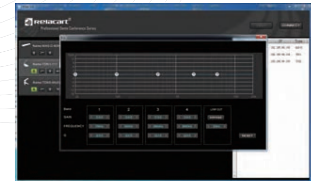
Some microphones support equalization adjustment function, 4-band equalization and high-pass filter can be set by software
